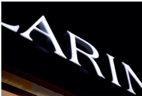
**MATERIAL** Lower part made of aluminium (painted in accordance with RAL or Sikkens Color Map solid), White undercoating inside Mirror 3 mm coloured acrylic and rear side clear acrylic
